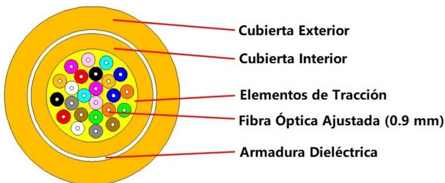
CABLE STRUCTURE AND PARAMETERS:
